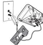
Align the holes on the bracket with the standard wall plate and slide the bracket down until it clicks securely in place.
